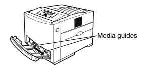
Insert media with the **printing side down** into the multi-purpose tray while adjusting the media guides to the media width.
